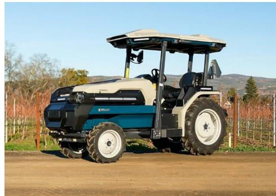
Due to limited onboard energy storage capacity, this equipment would be capable of approximately three hours of continuous operation, at which point the battery pack would be depleted. The vehicle design is such that the depleted battery pack is removed from the tractor and replaced with a fully charged battery pack. The depleted pack would then be connected to a battery charger.
