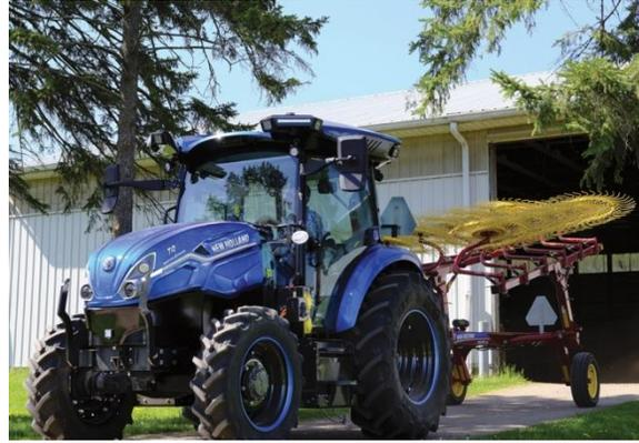
This equipment would require substantial modifications to the vegetation control operations currently employed at BUR. This vehicle would require a DCFC rated at greater than 120 kW. The operations scenario would include approximately three hours of equipment operation followed by one (1) hour of equipment fast charging.
